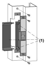
(1) If you order an ES2000X which has pre-drilled extension holes, 25 and 50mm extension lips can be fitted for extra wide door frames.
