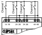
Be sure to tie the common terminals together when using this wiring style
