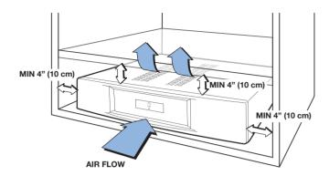
If the AKURATE amplifier has inadequate ventilation and/or is played very enthusiastically for a period of time, its temperature may rise above the designated operating level and the affected channels will shut down until they have cooled sufficiently.
